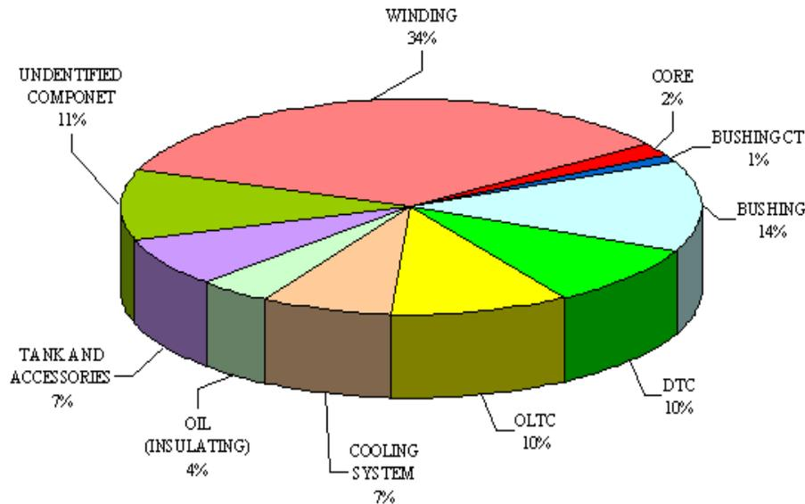
**Fig. 3 Number of transformer stoppages versus components**
